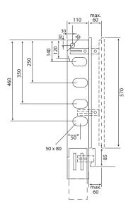
Flush mounted cabinets need a build-in hole, which is about 5 mm larger than the B measure and 600 mm above floor surface.
